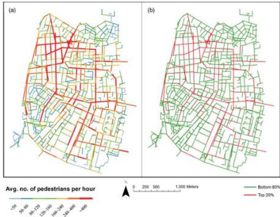
Figure 5. A visualization of the pedestrian movement prediction model for the current state of the city. (a) The full prediction amounts. (b) The strongest 20% of the street segments with regard to predicted pedestrian movement.
